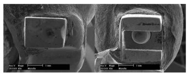
FIGURE 4. Stereomicroscope analysis for plastic insert precision attachment. White arrows indicate longitudinal grooves in patrix/matrix parts after 5 years of simulated use.
