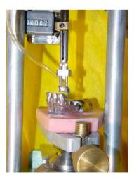
FIGURE 2. Insertion/removal cycling apparatus.
