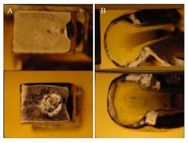
FIGURE 1. A) Plastic insert precision attachment, B) Metal-alloy precision attachment
